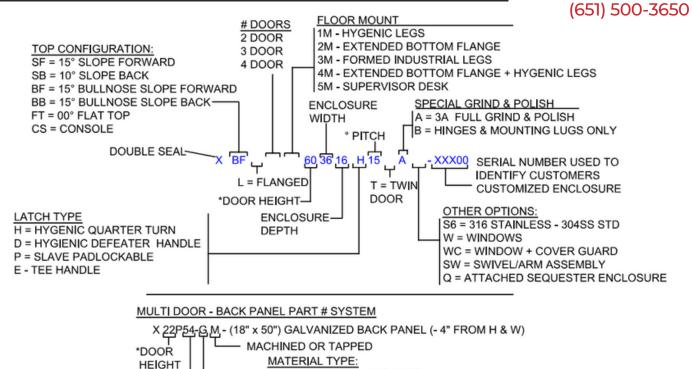
G - GALVANIZED - 12 GAUGE AL - ALUMINUM - 1/8" **ENCLOSURE** S - STAINLESS 304 - 12 GAUGE WIDTH
